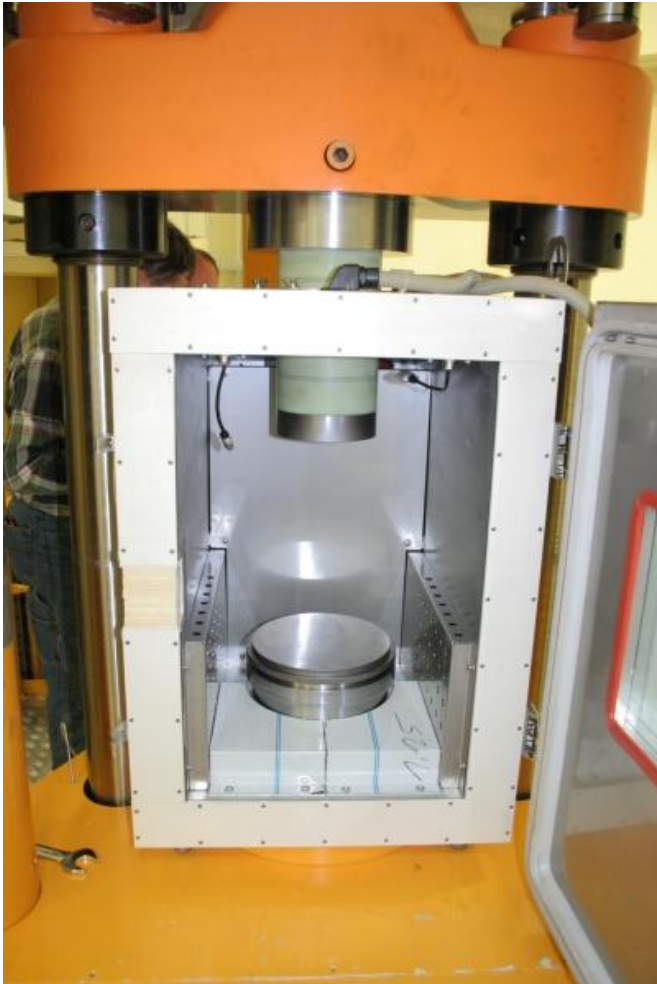
Climatic Chamber within the 2 MN Force Standard Machine
