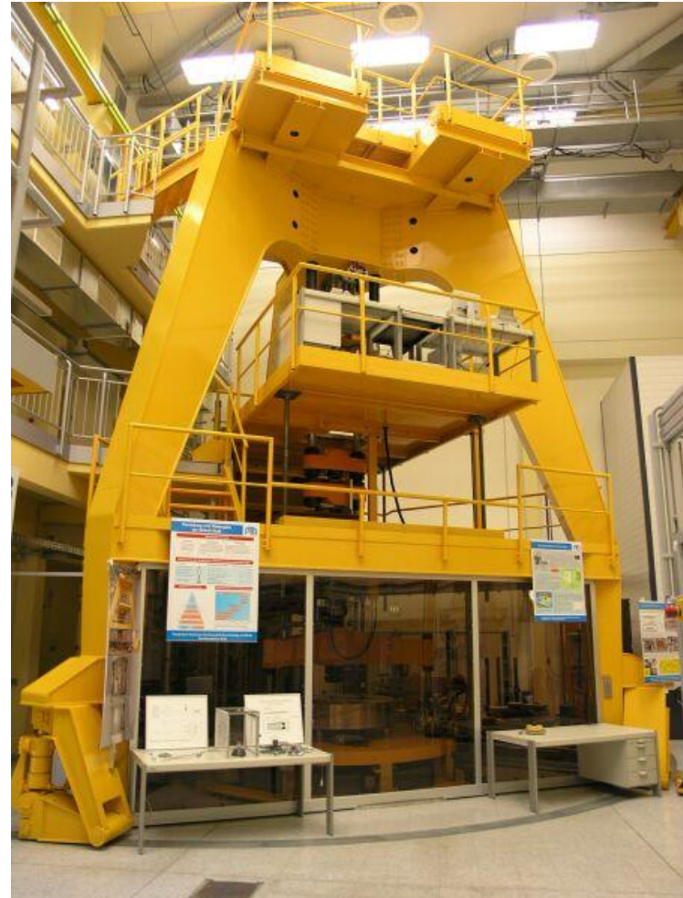
Climatic Chamber within the 2 MN Force Standard Machine
