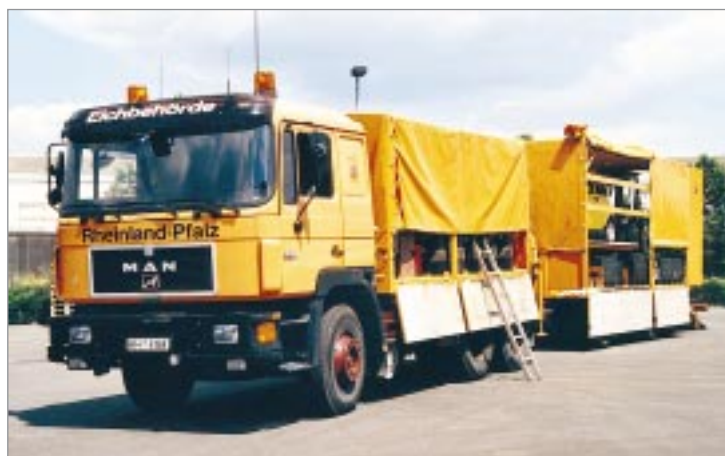
Fig. 1 Verification vehicle. On the tractor: 25 rolling weights (500 kg each); on the trailer: 15 t block weights, forklift and passenger car
