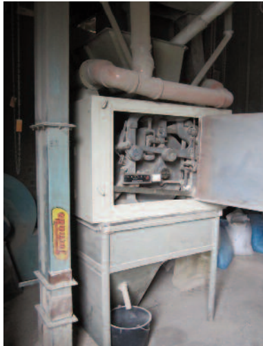
Chronos G 100 at the Demeter Biohof in Hennef-Dambroich (100 kg damping weight). Note that when closed (center picture) it can be locked by key to protect against unauthorized intervention.
