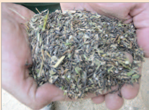
Fig. 5 Strip waste from the air separator
