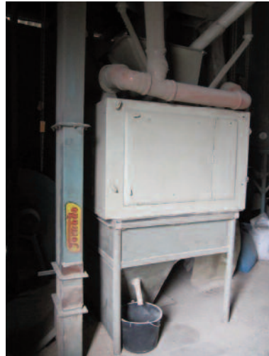
Chronos G 100 at the Demeter Biohof in Hennef-Dambroich (100 kg damping weight). Note that when closed (center picture) it can be locked by key to protect against unauthorized intervention.
