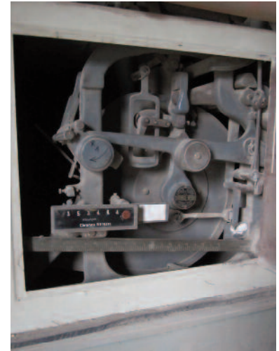
Chronos G 100 at the Demeter Biohof in Hennef-Dambroich (100 kg damping weight). Note that when closed (center picture) it can be locked by key to protect against unauthorized intervention.
