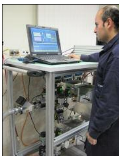
Figure 7 Critical flow nozzle bench in Peru
