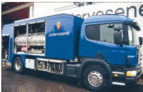
Fig. 1 Mobile calibration rig for volumetric testing
