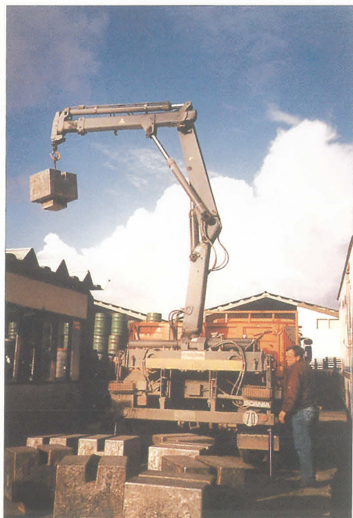
Fig. 3 Cubic standard weights lifted by using a crane.
