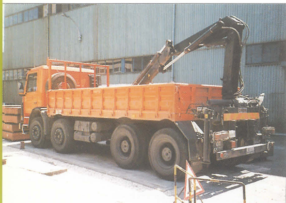
Fig. 2 The lorry used as a substitution load during the verification of a weighbridge in Portugal.
