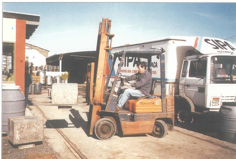
Fig. 4 Cubic standard weights lifted by means of a fork lift.
