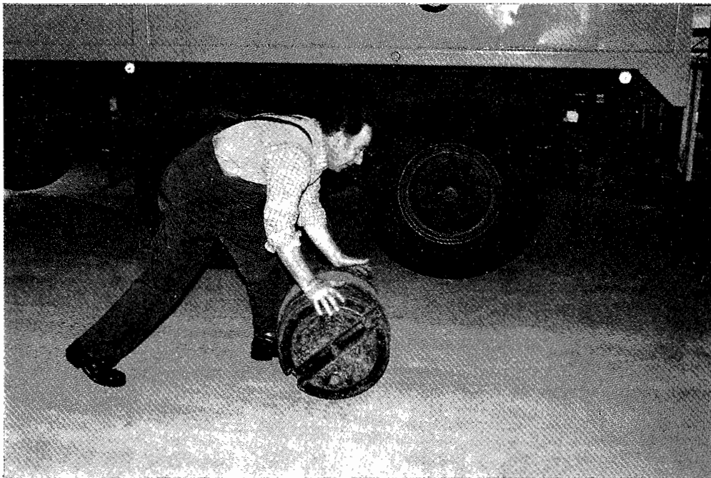
Fig. 2 — Handling of 500 kg standard weights on the ground without any device
