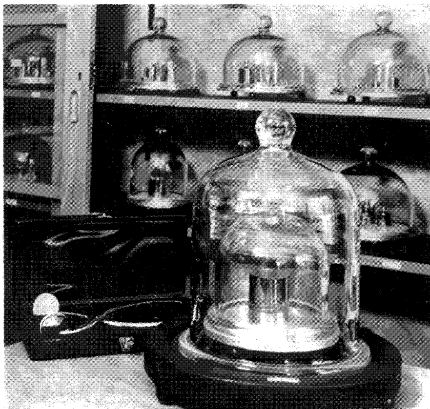
Fig. 1 National Kilogram Prototype N° 52, kept under two bell-jars. In the background, further primary and reference standards of the PTB.
